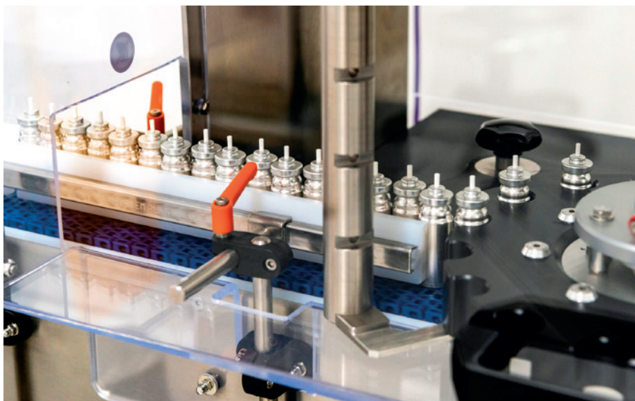
Figure 3: A semi-automated check-weigher, which enables a 100% check that all pMDI units are filled to the correct specification. Any out-of-specification pMDI units are automatically rejected.
