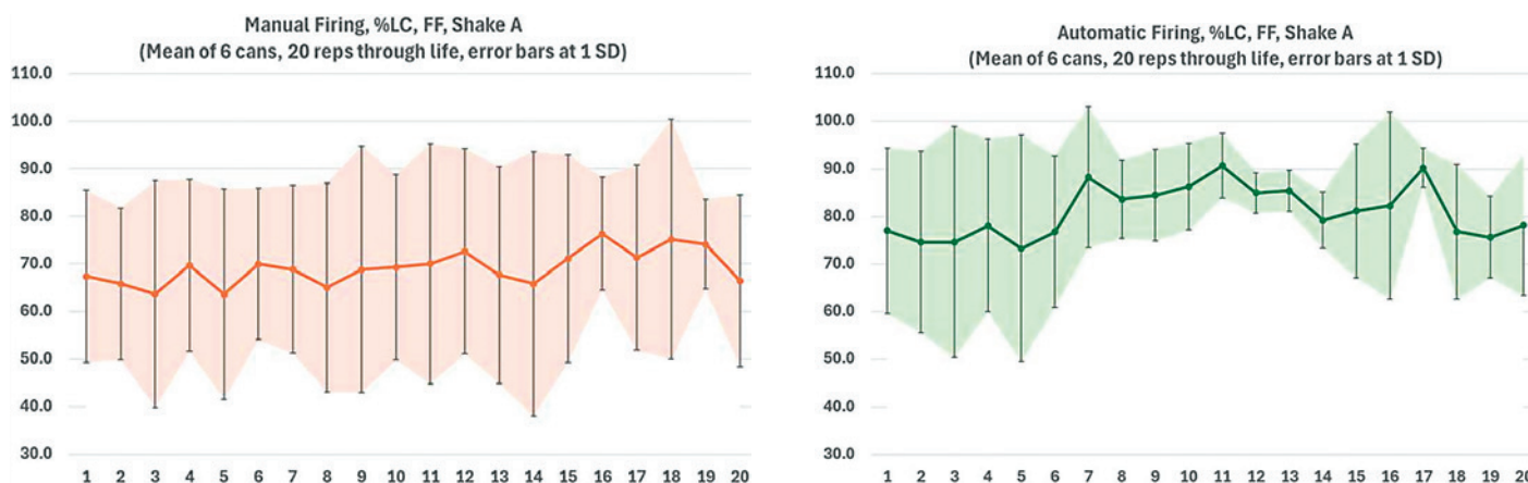
Figure 2: Under Shake A, automated actuation reduces the variability of the FF delivered dose relative to manual actuation, with tighter clustering around the mean. (Originally presented at DDL 2025 and reproduced with kind permission of the authors.)
