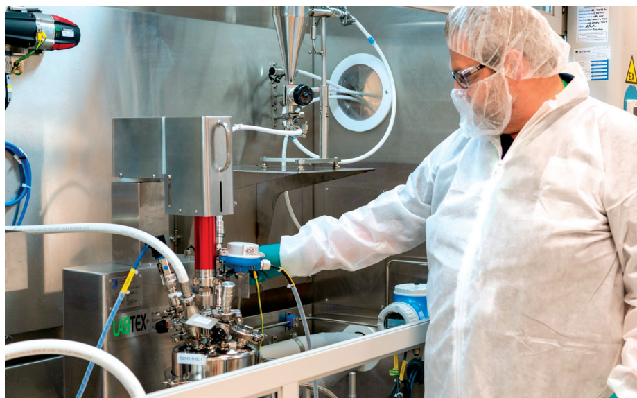
Figure 2: 5 L bulk suspension/solution manufacture with HFA-152a in ATEX-rated equipment.
