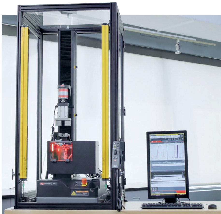
Figure 1: Instron Autoinjector Testing System, capable of full functionality testing for needle shield and button-activated devices, as well as safety syringes.
