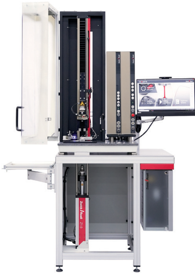
Figure 2: Testing autoinjectors without medication.
