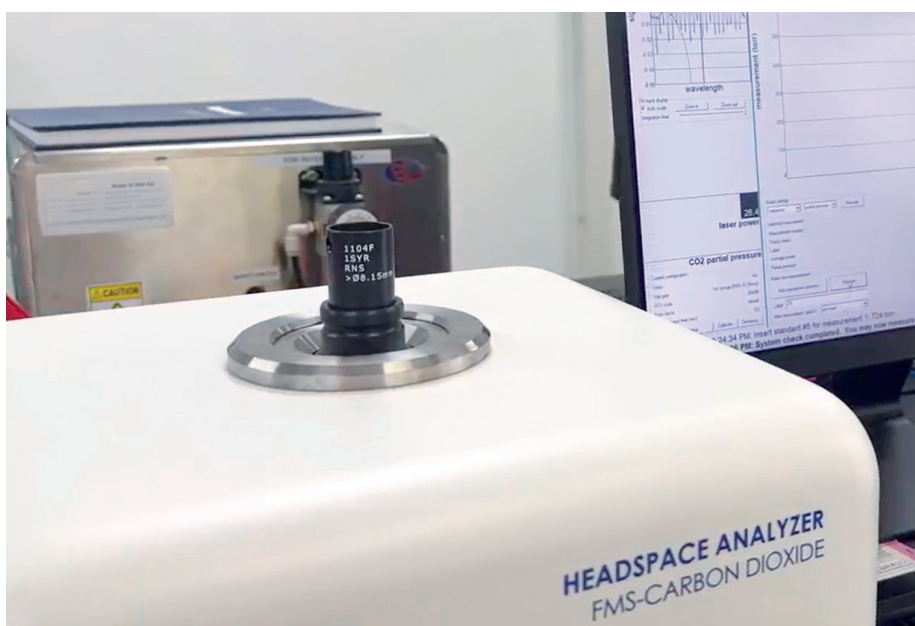
Figure 1: A laser headspace analyser at ZebraSci.
