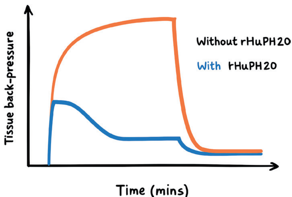
Figure 3: The effect of hyaluronidase adjuvant on the tissue back-pressure experienced during a 10 mL, 7 cP injection over several minutes. Note that the effect becomes apparent after a certain timescale during delivery and that a plateau is reached during the delivery. Reproduced from Pepin et al (2023).
