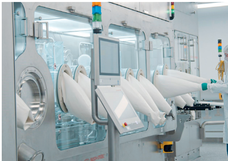
Figure 1: Specialist isolator technology may be required when filling highly sensitive biologics.
