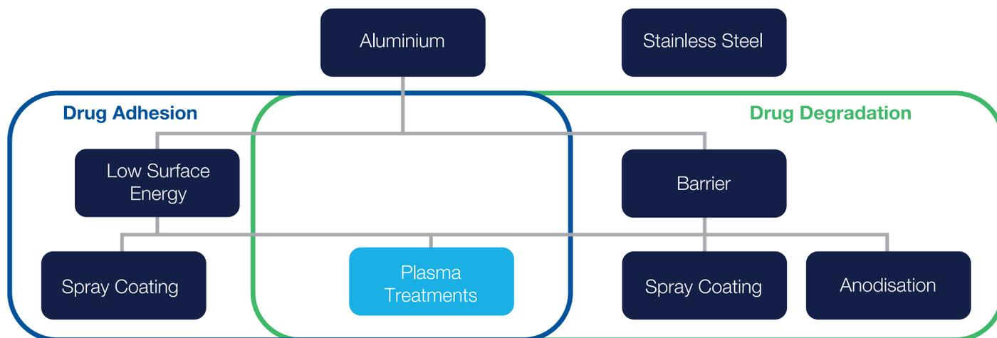
Figure 1: Types of surface treatment.
