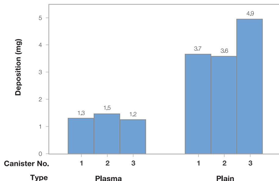
Figure 4: Drug deposition on canister walls after depletion of formulation.
