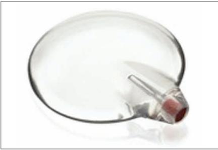
Figure 6: The primary drug container comprises a flexible multi-laminate blister heat-sealed to a rigid base plate, with integrated filling/discharge channel, sealed with a butyl rubber septum.
