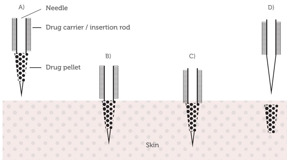
Figure 2: Sequence of microneedle delivery via the Micropatch™.
